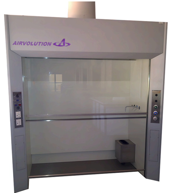
A Walk-in Fume cupboard connected to ducting
